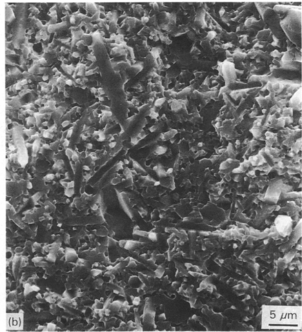
Figure 2 Scanning electron micrographs of fracture surfaces of sialon ceramic materials: (a) SA-1; (b) SA-2.
