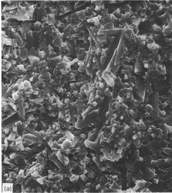
Figure 1 Scanning electron micrographs of fracture surfaces of silicon nitride ceramic materials: (a) SSN-1; (b) SSN-2.
