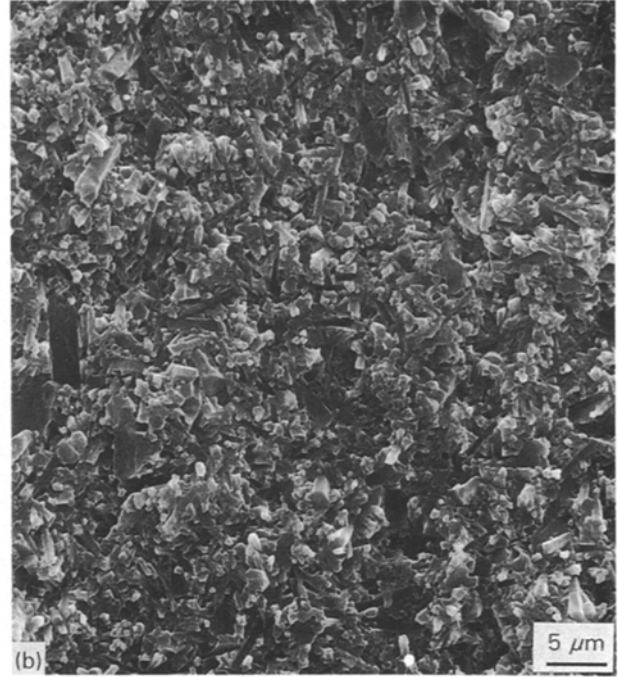
Figure 1 Scanning electron micrographs of fracture surfaces of silicon nitride ceramic materials: (a) SSN-1; (b) SSN-2.
